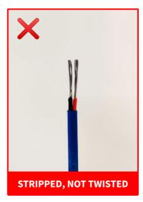
Remove insulation Twisting unexposed wires material and thoroughly will not make a connection and give measurement wires errors
